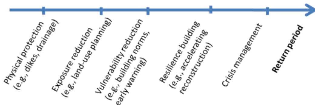
Figure 4: An example of risk-management policy mix, in which: (1) physical protections avoid frequent events, (2) land-use planning limit losses in these protections are overtopped, (3) vulnerability-reduction measures such as early warning and building norms minimize the direct losses from unavoidable disasters; (4) resilience-building measures minimize indirect losses from unavoidable disasters. Regardless of other measures, crisis management is always potentially needed to cope with the largest events that exceed the planned capacities.
